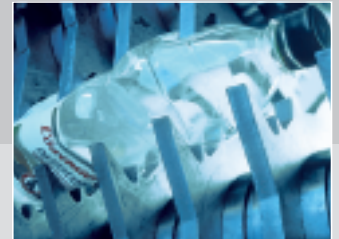
The special shape of the rollers - with large and small grippers - ensures reliable feeding of varying bottle sizes.
