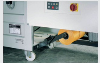
Convenient and firm strapping of the bales thanks to sophisticated strapping technology with polyester tape.
