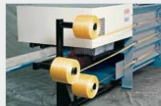
Bales are strapped easily and tightly with polyester tape through the use of proven strapping equipment.
