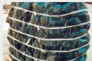
Optimum compression result with difficult materials, e.g. car tires on europallet.
